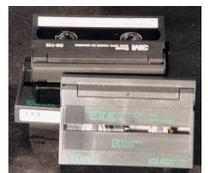
Exabyte tapes come in 2 densities: 5Gb (read by the EXB-8205 drive) and 10Gb (read by the EXB-8505 drive). Picker only uses the low density for their IQ/PQ tapes.
