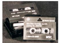
DAT drives come in 3 densities: standard (DDS), double (DDS-2) and quad (DDS-3) density. To our knowledge, GE only uses the standard (DDS) density.
