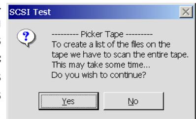
In some cases, when readOmatic has to scan the entire media, it will offer you the possibility of reading and saving the media content while it scans. This possibility is only offered for a few tape formats. Since the content structure is not known yet, the files saved with this option will all be in the same directory (the subdirectory “readOmatic” in your scratch file directory) without any subdirectory for studies or series.
